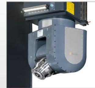
• High Precision (Positioning Accuracy  $\pm 5\mu\text{m}$ ) Kessler 2-axis Head
