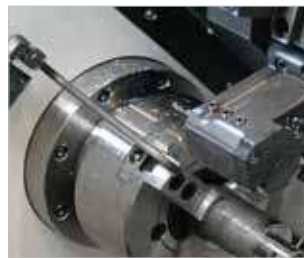
Chuck Air Blow (Upper Chuck)
