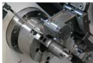
Chuck Air Blow (Upper Chuck)
